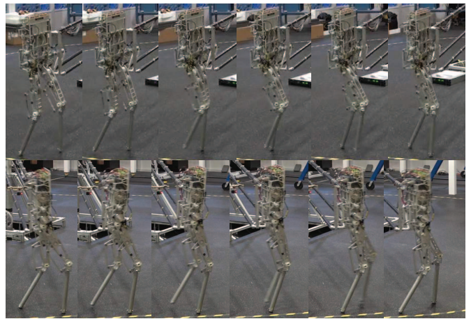
Fig. 3. Snapshots from experimental implementation of the two gait design methods on AMBER-3M. (Top) An Implicit Mechanics-Based gait produced by the methods described in Section III. (Bottom) An optimized gait with mechanics-based constraints produced by the method in Section IV.
