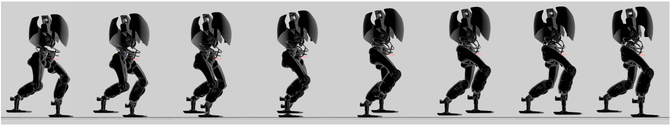
Fig. 8: Tiled still images the DURUS running at 2.0 m/s.
